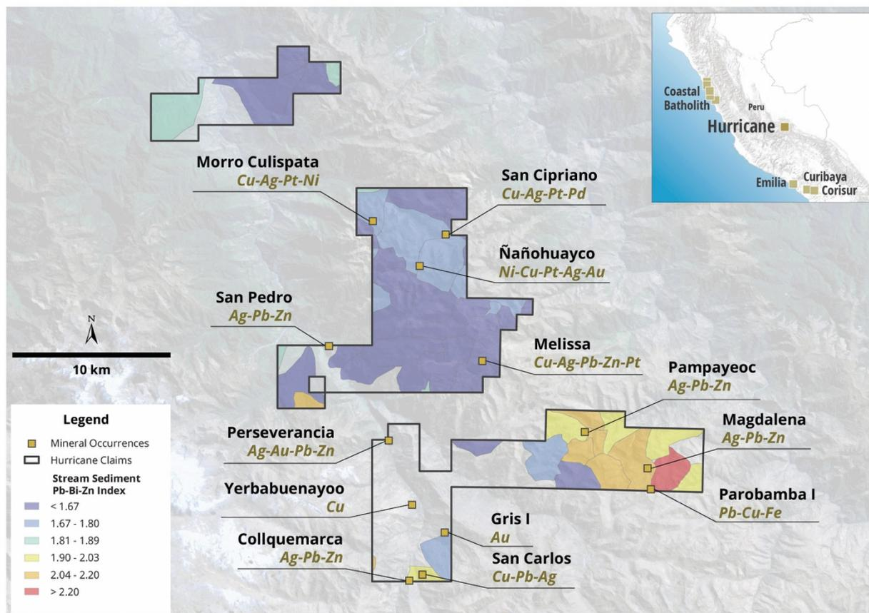
Figure 6: Illustrates lead-bismuth-zinc anomalies in drainage basins that are interpreted to be associated with intermediate sulphidation styles of mineralization.
